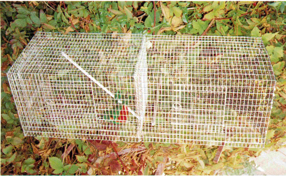
This special devise looks like a bird cage but is, in fact, an excellent bird trap. It has two sections. One contains a decoy bird while the escapee can enter the other through a wire funnel.
