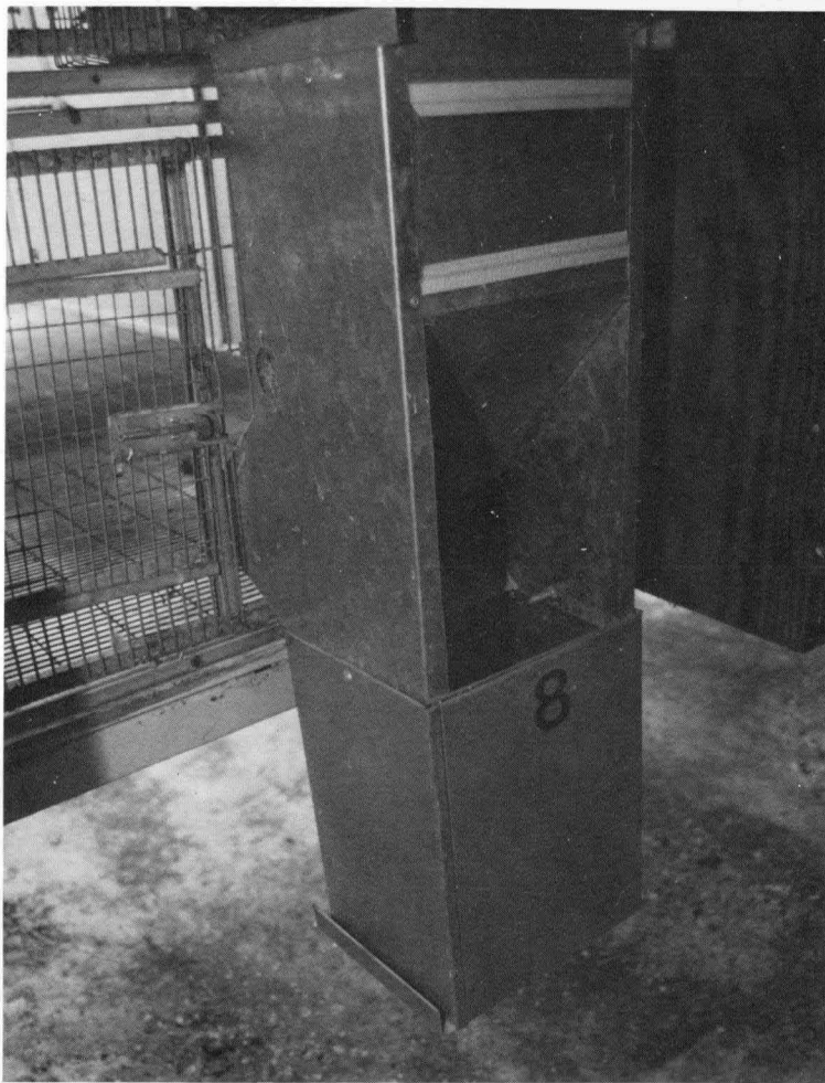
This rear view of seed hopper shows the spilled and wasted seed retrieval bin on the bottom of the hopper.
