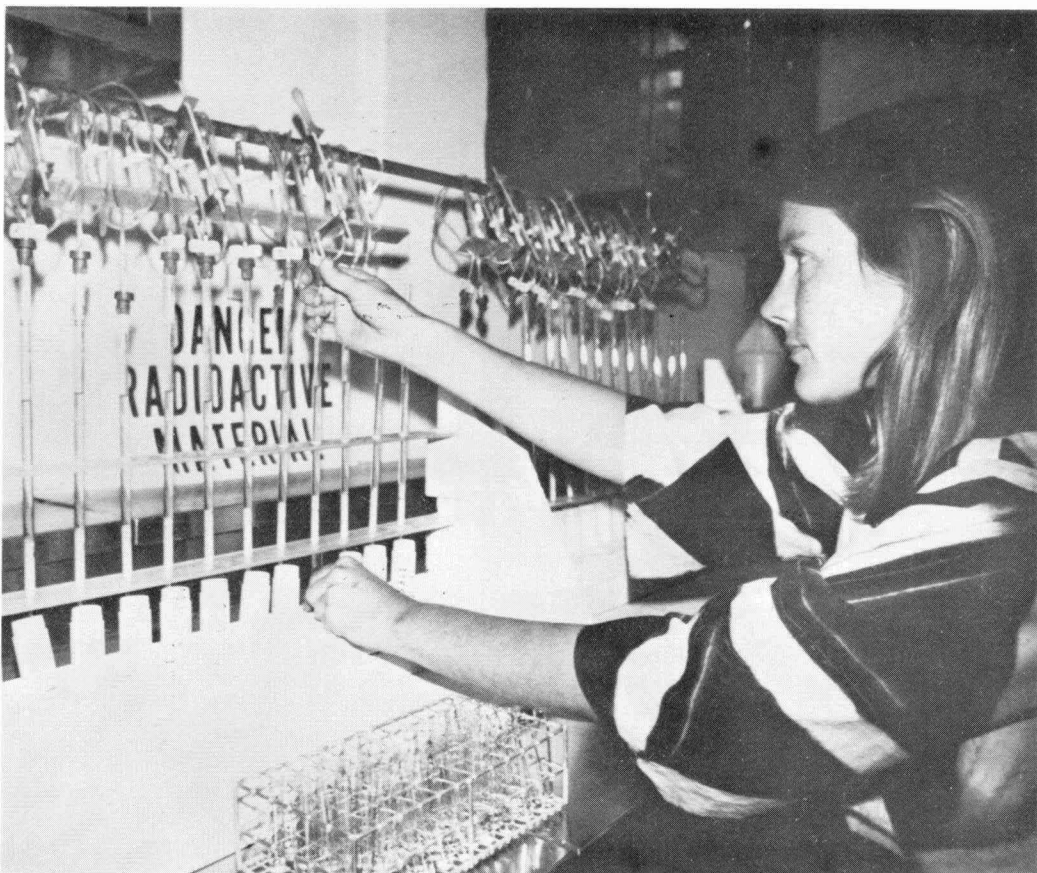
Laboratory technician prepares column apparatus for separation of steroids from fecal sample.
