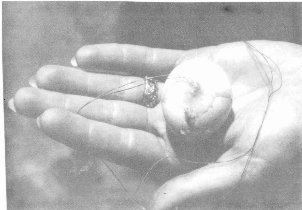
Thermocoupler implanted in infertile egg by researcher, Don Hoyt, UCLA graduate student.
